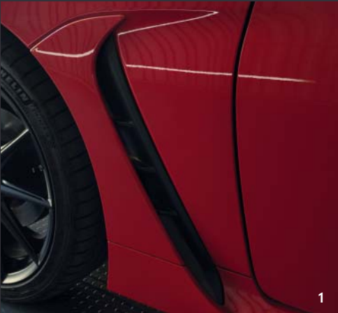
1. Informed by Toyota motorsport innovation, GR86 is fitted with front air outlets which allows air inside the front wheel arch to escape, enhancing excellent steering stability. 2. Muscular, wider rear profile enhances stability.
